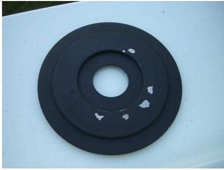
triggerplate from RB80 with unique defect coat
