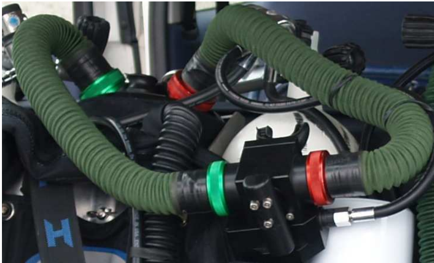
Cooperhoses with OC-Mouthpiece, on the OC-Mouthpiece is on 2 nd stage one Apeks FreeflowDevice
