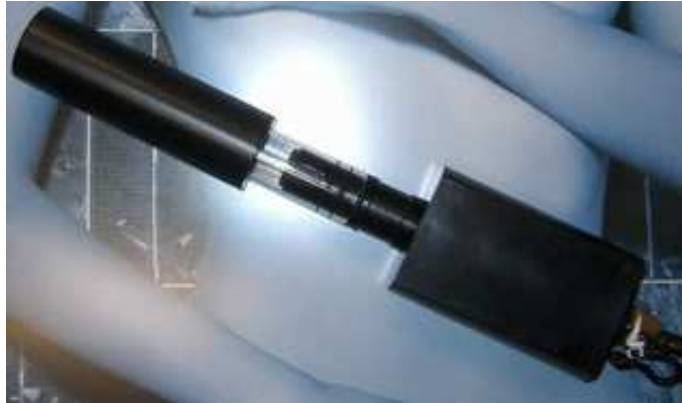
ProtectionTube is on one 24W HID Lighthead
