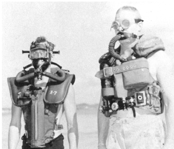
Figure 7. The LARU-X and the Amphibian Mark II (CJL photo).
