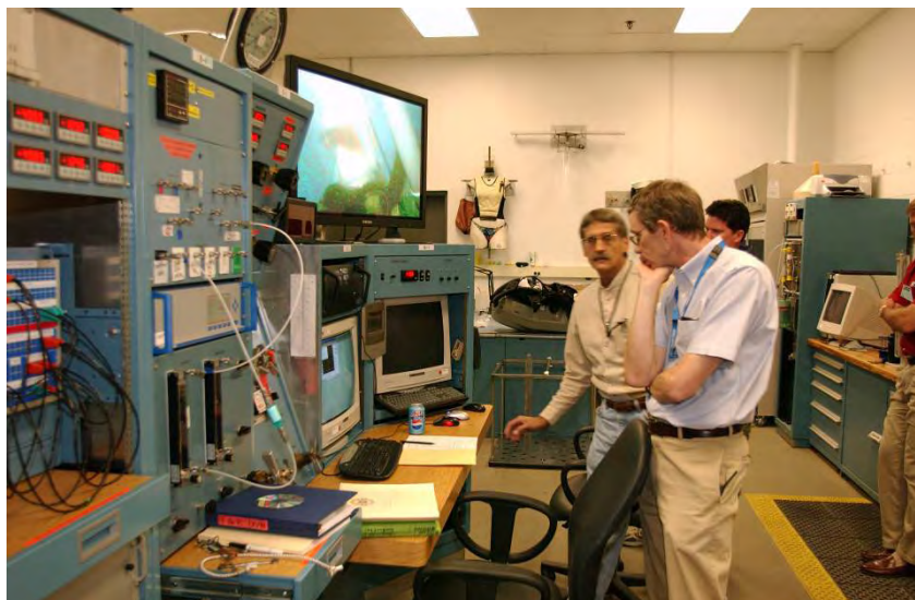
Figure 8. Control console for unmanned equipment testing.
