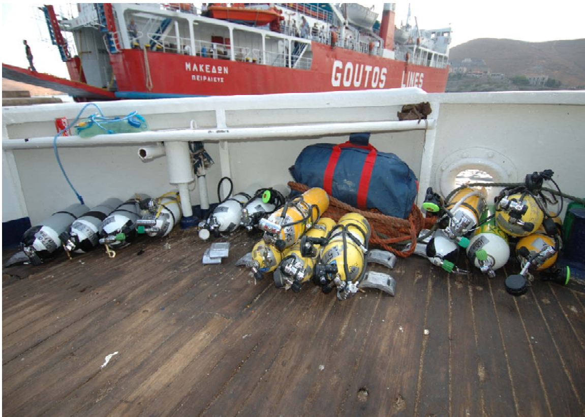
Figure 5. Gas supplies for open circuit bail-out (Richie Kohler).
