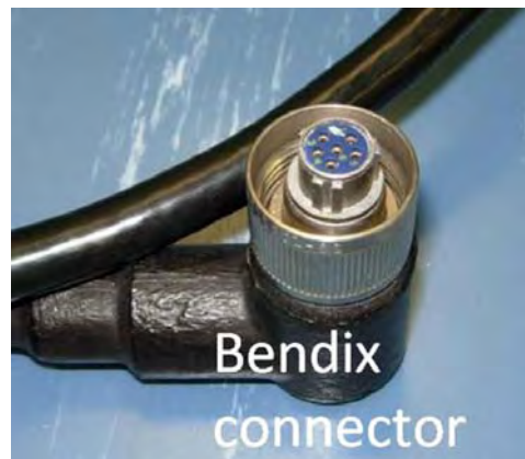
Figure 19. MK 16 Bendix connector.
