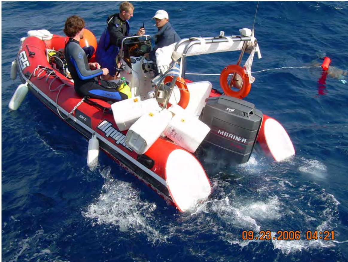
Figure 8. Surface attendants in the RHIB with buoys, lines and reserve gas for decompression (PJD).
