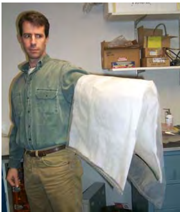
Figure 3a: Aspen Aerogel Cloth Super-Insulation
