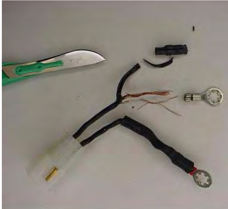
Figure 22. Connecting wires damaged by improper repair.
