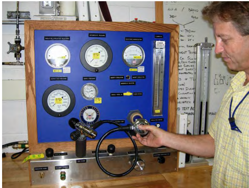
Figure 3. NEDU’s scuba regulator dry test bench and NEDU lead Investigator for Diving Accidents, David Cowgill.
