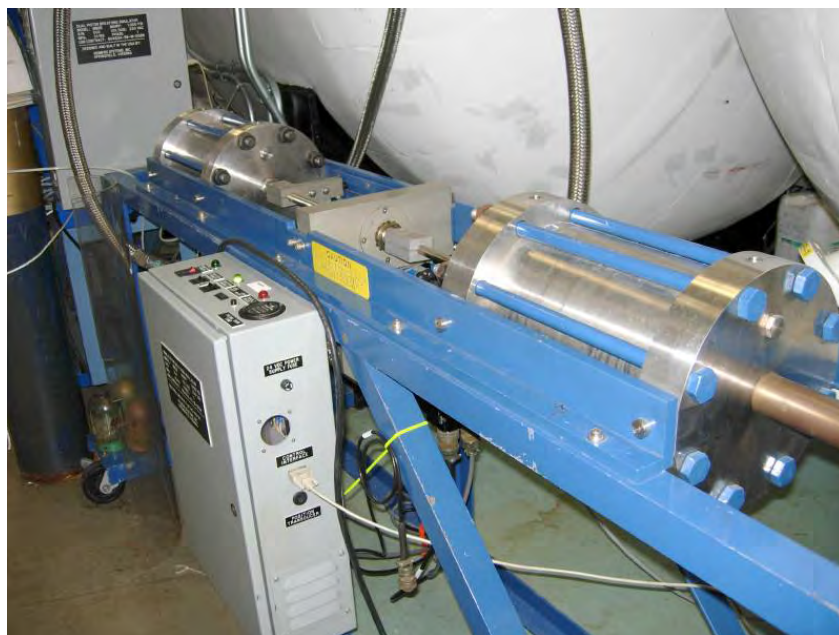
Figure 9. Dual-headed breathing machine used to simulate two divers breathing on two UBA simultaneously.
