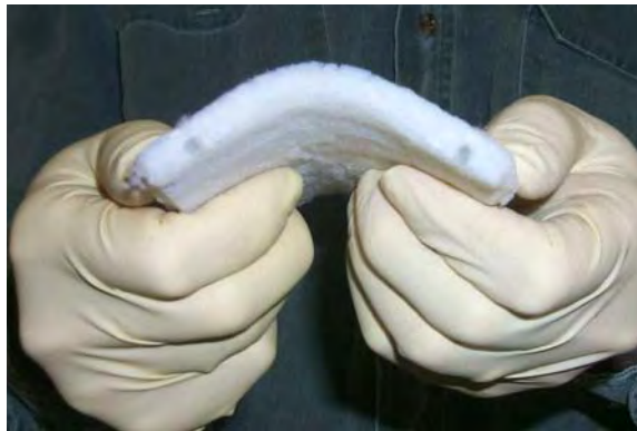
Figure 3b: Aspen Aerogel Cloth Super-Insulation
