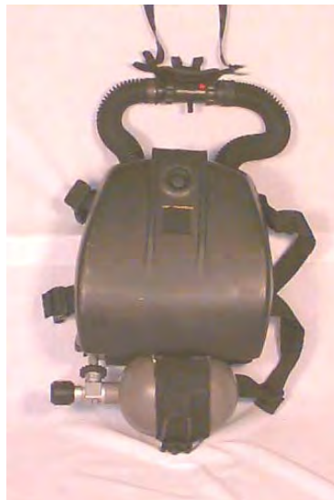
Figure 12. A LAR V Nitrox (LAR VII) semi-closed UBA.
